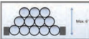
Stacking pipe for temporary storage
