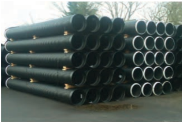
18" pipe stored in 20 piece bundles
