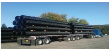
18" and 24" StormTite™ Plain End Pipe, 30' length
